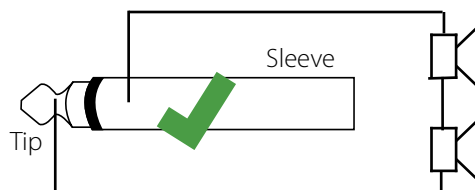
Correct mono plug wiring - speakers in series
